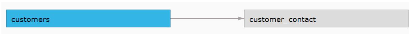
Figure 7. Restructured CustomerContact entity and reversed relationship to hold the pivoted data set
