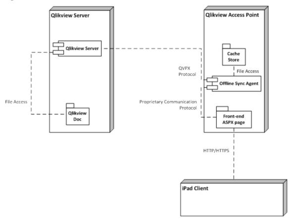
This is the high level architecture of the solution. The client requests offline documents via a new "Offline service" that does the job of preparing a cache with data slices. These data slices are then pulled from the client for offline use.
