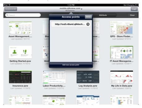
3. You cannot remove the Access Point that you are currently using. First, you must navigate to the new Access Point, then you can remove the prior entry. Setting up a new Access Point requires that you enter the AP URL (omit the '/qlikview' part) e.g. demo.qlikview.com.
