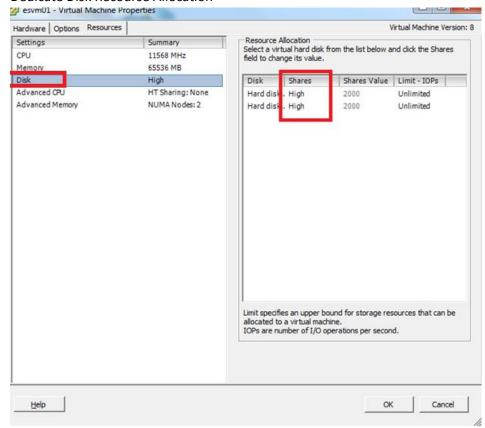
• Change Advanced CPU Hyper threading > set to None
