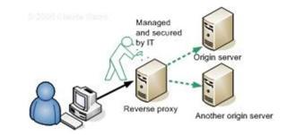
É A reverse proxy is either a proxy server that is installed in a server network or a network equipment.
